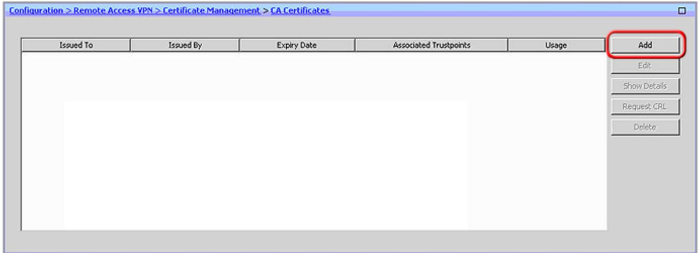
3. Assign a 'Trustpoint Name' to the certificate (e.g. DigiCertCA2), And select the 'Install from a file' Radio Button and browse to DigiCertCA2.crt. Then click 'Install Certificate'. Then repeat this process of adding a new trustpoint and installing the certificate file for 'DigiCertCA.crt'.
